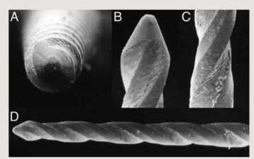
**2.5** Axial **(A)** and side **(D)** views and details of the tip **(B)** and blade **(C)** of the Quantec SC instrument, observations made with SEM (Scanning Electron Microscope) between 600X and 500X.
