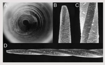
**2.7** Axial **(A)** and side **(D)** views and details of the tip **(B)** and blade **(C)** of the ProFile instrument, observations made with SEM (Scanning Electron Microscope) between 60X and 500X.
