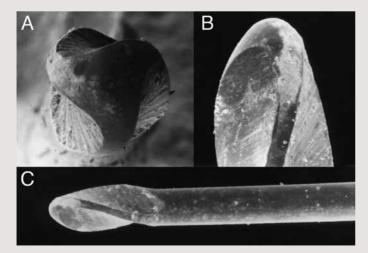
**2.6** Axial **(A)** and side **(C)** views and details of the tip and blade **(B)** of the LightSpeed instrument, observations made with SEM (Scanning Electron Microscope) between 60X and 500X.
