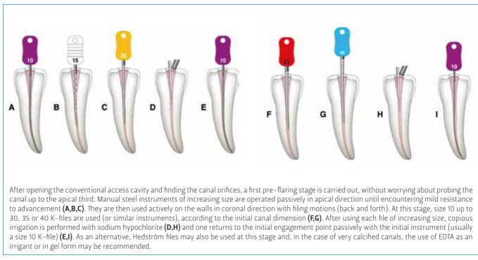
**2.1** Scianamblo and Ruddle technique for the preparation of root canals, one of the most advanced techniques for shaping and cleaning root canals before the introduction of NiTi instruments.
